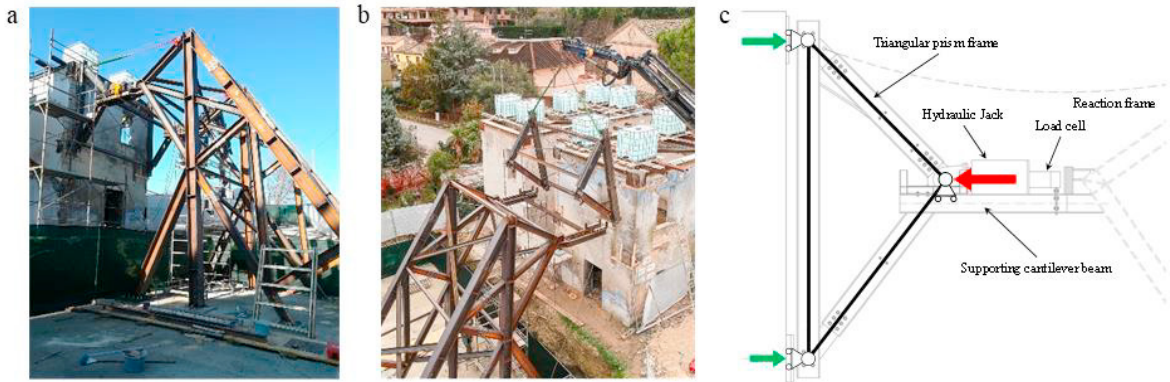
Fig. 3. (a) Pushing system during the test; (b) Assembly of the triangular steel frame; (c) Static scheme of the triangular steel frame.
